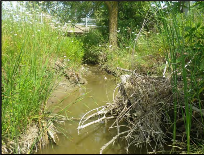
29. Reach C-7: woody debris has caused constriction of flow and local increase in erosion
