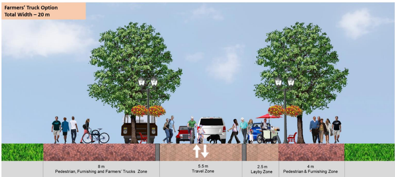
FIGURE 5-2: PROPOSED CONCEPT - SHARED STREET CROSS-SECTION WITH ADDITIONAL SPACE FOR FARMERS’ TRUCKS
