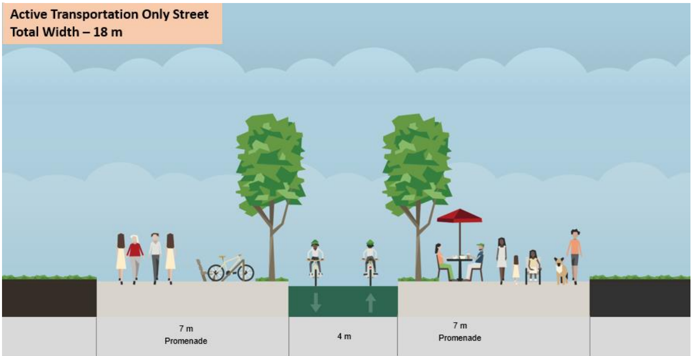
FIGURE 5-6: PROPOSED CONCEPT – ACTIVE TRANSPORTATION CONNECTION CROSS-SECTION
