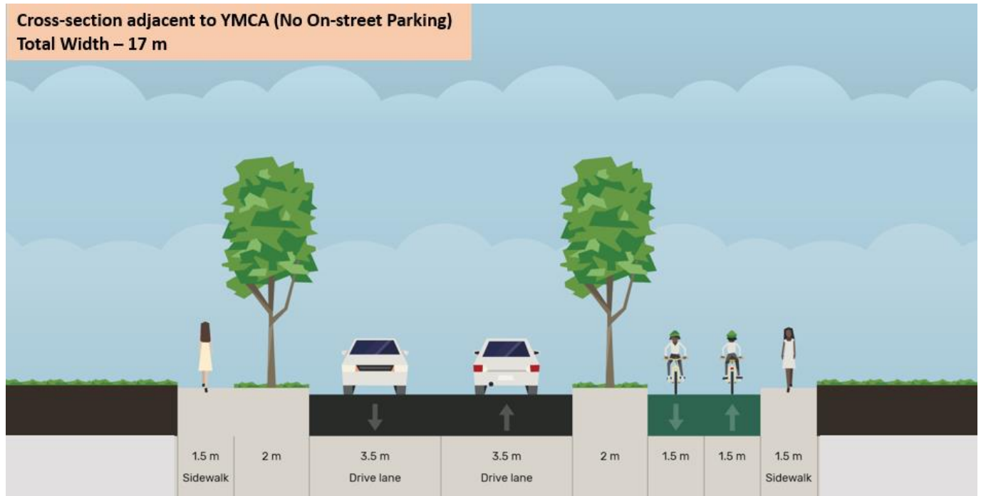
FIGURE 5-7: PROPOSED CONCEPT – CONVENTIONAL MULTIMODAL STREET CROSS-SECTION
