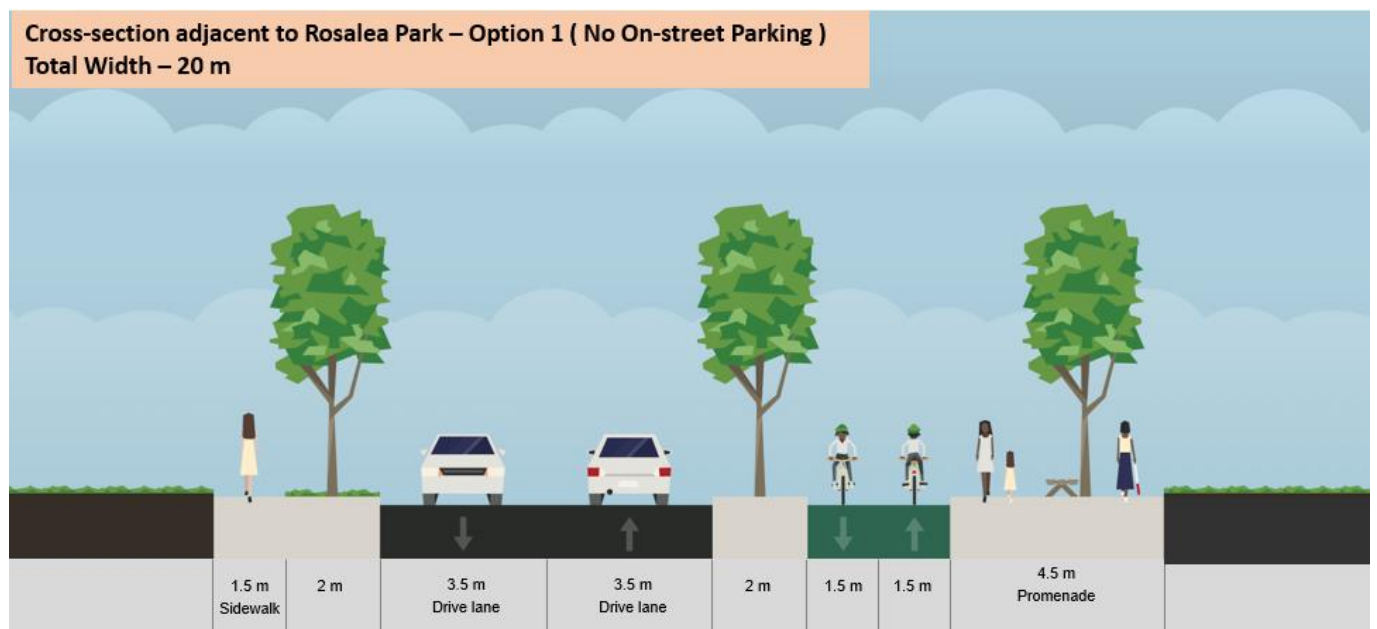
FIGURE 5-8: PROPOSED CONCEPT – CONVENTIONAL MULTIMODAL STREET CROSS-SECTION
