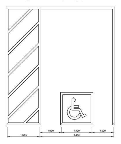
3. The following diagram illustrates the location of the pavement markings within a Type B, accessible parking space.
