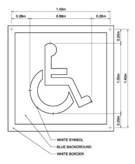
2. The following diagram illustrates the location of the pavement markings within a Type A, accessible parking space.
